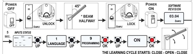
➡ If the operator performs the first learning cycle starting in opening, wait for the end of the cycle and reverse the motor rotation through the menu 5, then repeat the learning procedure
