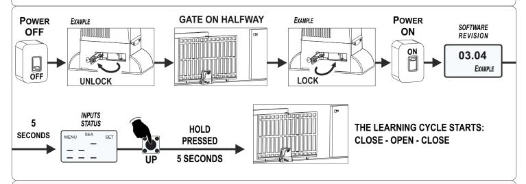
□ If the operator performs the first learning cycle starting in opening, wait for the end of the cycle and reverse the motor rotation through the menu 5, then repeat the learning procedure
