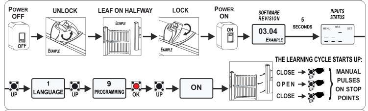
If the operator performs the first learning cycle starting in opening, wait for the end of the cycle and reverse the motor rotation through the menu 5, then repeat the learning procedure
