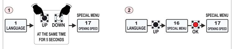
IN THE **BASIC MENU** IT IS POSSIBLE TO **SELECT THE OPERATOR TYPE** IN USE AND OTHER NECESSARY OPTIONS. ONCE THE TYPE HAS BEEN CHOSEN, ALL THE SPECIAL MENUS ARE AUTOMATICALLY SET TO THE DEFAULT VALUES USEFUL FOR THAT OPERATOR, SO FURTHER SETTINGS MAY NOT BE NECESSARY
